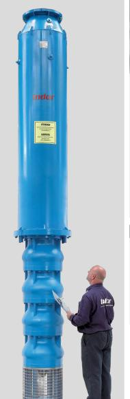
The INDAR SP **UGP** series consists of submersible pumps and motors designed for pumping clean or slightly contaminated water in a wide range of sectors and applications. INDAR **UGP** pumps are multistage centrifugal pumps directly coupled to an INDAR submersible electric motor designed for permanent submersible operation. All parts of the pump and the motor are completely designed and manufactured by INDAR in Spain.
